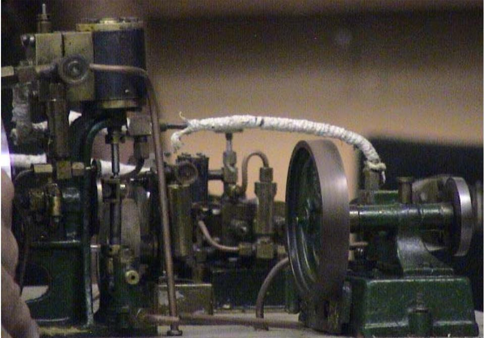
The above photo shows a collection of engines mounted on a board. Each engine had air supply piping and all are connected to a central feed point via valves. The setup allows each individual engine to be run as required at an exhibition for demonstration purposes, (or pleasure). The assembly has been left to the society by a deceased member. It was said that this item had been exhibited at Barnet college about 20 years ago.
